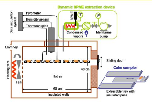
Figure 9: Diagram of the Reactial oven for monitoring the CNFV during cooking. According to the thesis of S. Fehaili (*Th1*).
