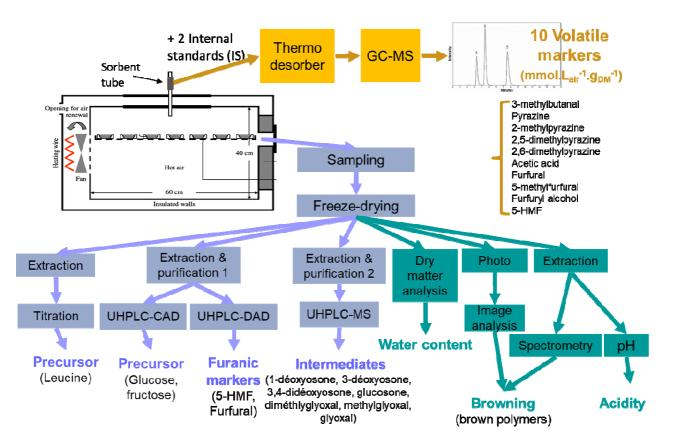
Figure 12: Analytical strategy of 20 volatile and non-volatile markers for monitoring reactivity in a model sponge cake. According to (Oral1).
