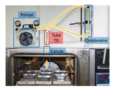
Figure 10: Diagram of the extraction assembly using on-line adsorbent tubes suitable for the Reactial baking oven. According to (Poster12).
