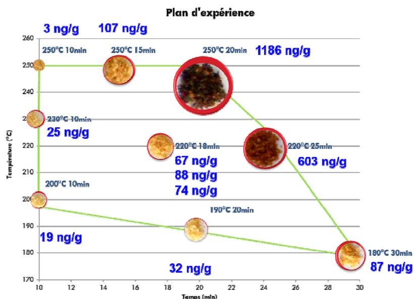
Figure 22: Furan concentration (ng/g of product on a dry basis) determined in "oven fries" cooked according to the experimental plan of the Dominove project. The lower boundary of the experiment plan (200°C/10 min) corresponds to the setting cooking conditions. Dosage by isotopic dilution and standard additions. HS extraction coupled with GC / MS analysis in SIM mode.
