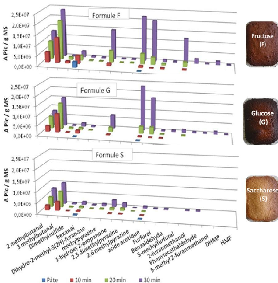
Figure 18: Evolution of the main CNFV for 3 formulas based on different sugars (F: Fructose, G: glucose; S: sucrose) according to the cooking time at 170 ° C. HS-SPME extraction with DVB / Car / PDMS fiber. According to (*Mast7*).
