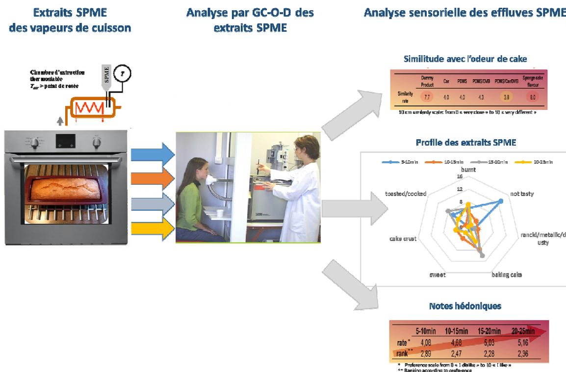
Figure 6: Schematic of the work on sensory & analytical optimization of the SPME extraction of key compounds of the gourmet aroma of "sponge cake" which is released when sponge cake is cooked.
