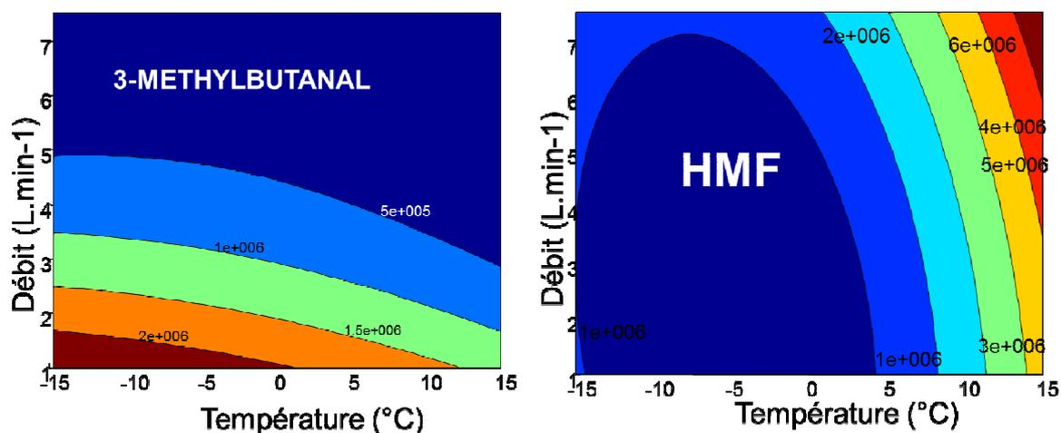
Figure 7: Response surfaces of 3-methyl butanal and of HMF extracted by dynamic SPME and analyzed by GC / MS in SIM mode. The red areas are most favorable for the dynamic extraction of the compound. According to M. Maire's defence (Mast5).
