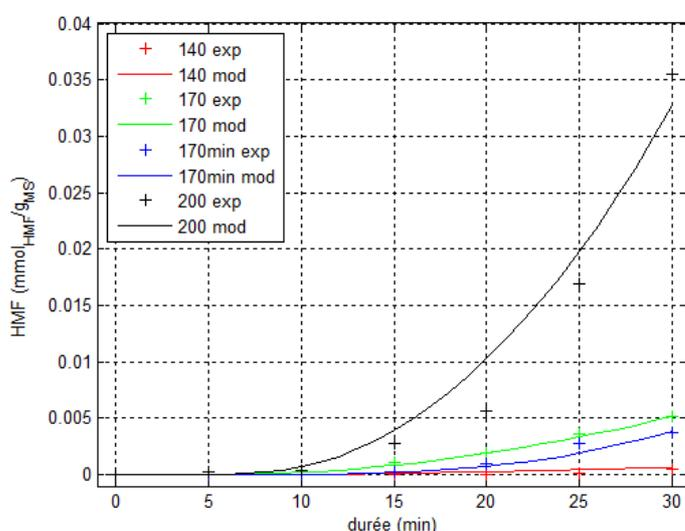
Figure 31: Tentative model of HMF production using zero order kinetics. Calculations were made by my colleague Bertrand Heyd under Matlab.
