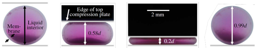
Figure 5. Side-view images of a capsule under the axial compression in a saline solution. After removing the top plate, the capsule has returned to its undeformed shape. Adapted from Ref. [54].
