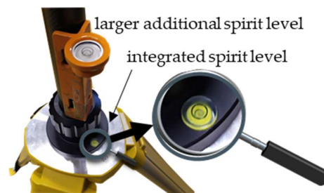
Figure 13. Larger additional spirit level added to the D-RTK2 tripod.
