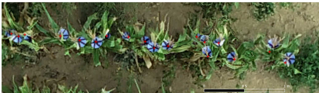
Figure 28. Final ortho-mosaic of R_1 reconstruction, visualized in the QGIS software, zoom on the second maize row, with in overlay the plant positions, measured on the ground with Geo7x DGNS in pole mode (+).
