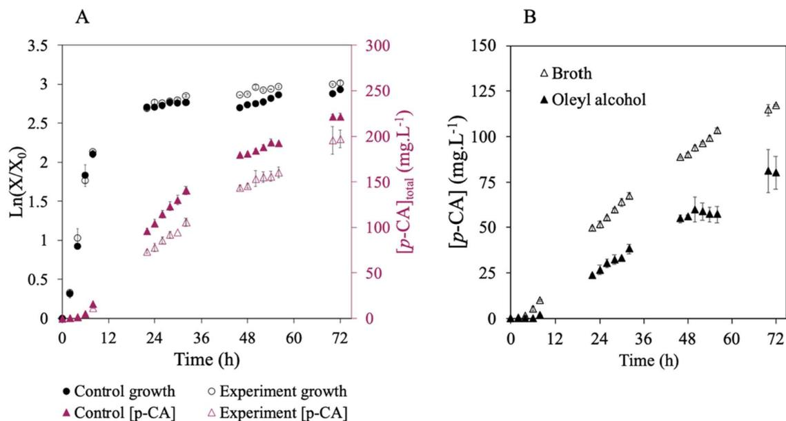
**Fig. 4.** A: Growths and *p*-CA total concentrations in control and extractive fermentations/experiment ( $[p\text{-CA}]_{\text{aq}} + [p\text{-CA}]_{\text{org}}$ ). B: Distribution of *p*-CA in the extractive fermentation.
