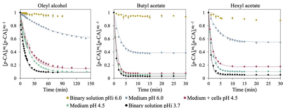
**Fig. 2.** Dimensionless  $p$ -CA concentrations in the aqueous phase in function of time through HFMC-assisted LLE with three solvents. Lines correspond to applications of the function in equation (4) for aqueous content of  $p$ -CA with respective  $\tau$ .
