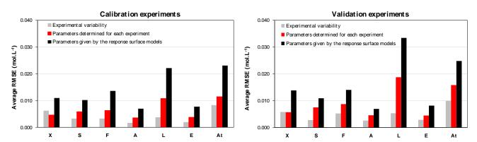
**Figure 7.** Comparison between experimental variability and average RMSE values for concentrations computed using parameters determined for each experiment (Table 2) and the response surface models (Table A2 and Equation (17)).
