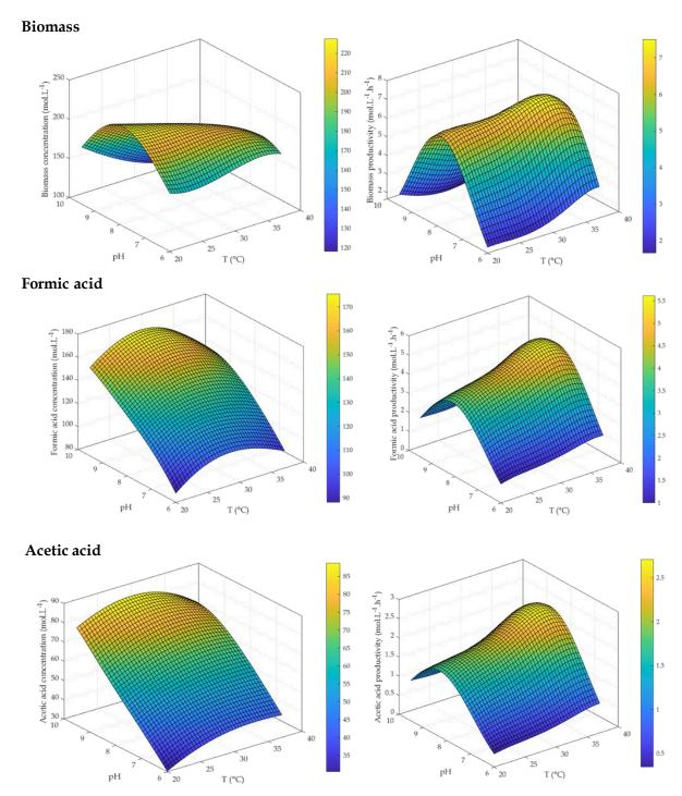
**Figure A2.** Evolution of final concentrations (left) and batch-average productivities (right) with temperature and pH for biomass, formic acid, and acetic acid.
