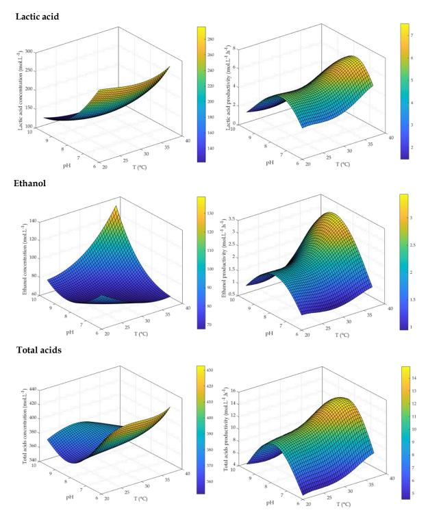
**Figure A3** Evolution of final concentrations (left) and batch-average productivities (right) with temperature and pH for lactic acid, ethanol, and total acids.
