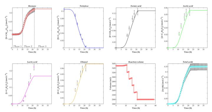
**Figure 5.** Evolution of concentrations over time for experiment F10 (T = 30 °C, pH = 8). Comparison between model (continuous line, using parameters from Tables 1 and 2) and experimental data (symbols). The error bars for data represent the biological standard deviation, calculated from three independent repetitions of the run F01.
