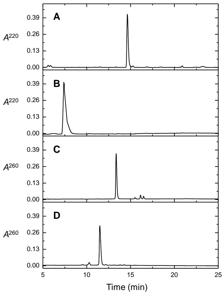
**Figure 2. HPLC characterization of pantathine conversions. A. Pantethine 8. B. Phosphopantethine 9. C. Dephospho-coenzyme A disulfide 10. D. Disulfide-coenzyme A 11.**
