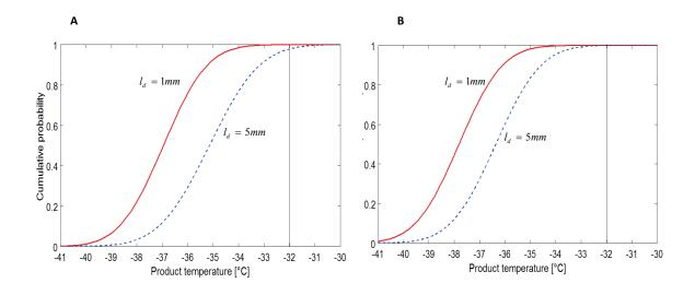
**Fig. 10:** Cumulative probability distributions of the product temperature obtained for freezedrying cycles carried out with spontaneous nucleation (S5) (Fig. 9A) and without controlled nucleation (S5cn) (Fig. 9B). Solid and dotted lines represent the product resistance distribution at 1 mm and 5 mm respectively. Vertical lines represent the critical product temperature (-32°C for sucrose).
