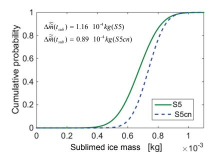
**Fig. 8:** Cumulative probability of the water mass loss determined from data obtained by using the gravimetric method in cycles performed with spontaneous nucleation (S5, dotted line) and controlled nucleation (S5cn, dashed line). The standard deviation of the mass loss for the two sets of data is reported on the figure.
