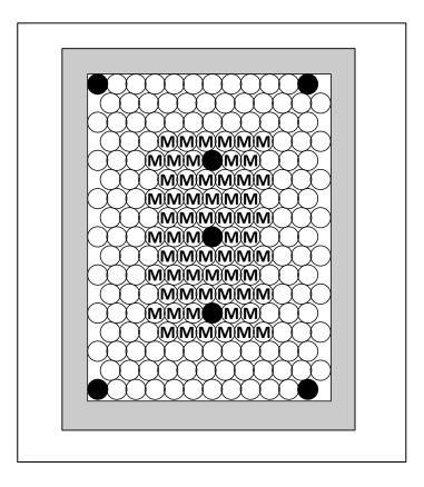
**Fig. 1:** Arrangement of the vials on the shelf. Symbols: black circle, vials in which the thermocouples are located; Letter 'M', gravimetrically-analyzed vials. All vials were filled with 1.8 mL of the selected product.
