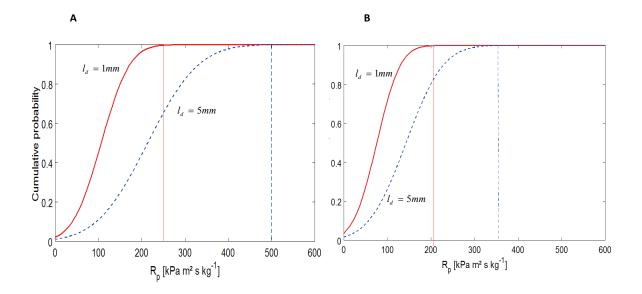
**Fig. 9:** Cumulative probability distributions of the product resistance obtained from the set of parameters obtained with spontaneous nucleation (S5) (Fig. 8A) and with controlled nucleation (S5cn) (Fig. 8B). Solid and dotted bold lines represent respectively the product resistance distribution at 1 mm and 5 mm. Vertical lines include approximately 99 % of values of the product resistance.
