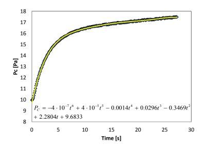
**Fig. 3:** Example of the increase of the chamber pressure in time during a pressure rise test (PRT) performed during the freeze-drying cycles S5-1 (spontaneous nucleation).
