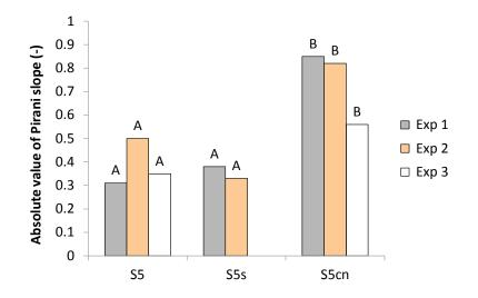
**Fig. 5:** Absolute value of Pirani slope at the end of sublimation obtained from freeze-drying cycles performed with product processed in vials without stoppers and spontaneous nucleation (S5), with partially inserted stoppers and spontaneous nucleation (S5s) and without stoppers and with controlled nucleation (S5cn). Experiments marked with the letter A in the legend show a significant difference at 0.05 level than experiments marked with the letter B (ANOVA test).
