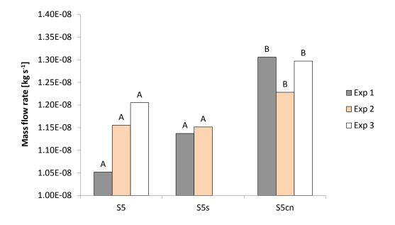
**Fig. 6:** Average values of the mass flow rates within a range of dried layer thickness between 0.5 mm and 7 mm in case of product processed in vials without stoppers and spontaneous nucleation (S5), with partially inserted stoppers and spontaneous nucleation (S5s) and without stoppers and with controlled nucleation (S5cn). Experiments marked with the letter A in the legend show a significant difference at 0.05 level than experiments marked with the letter B (ANOVA test).
