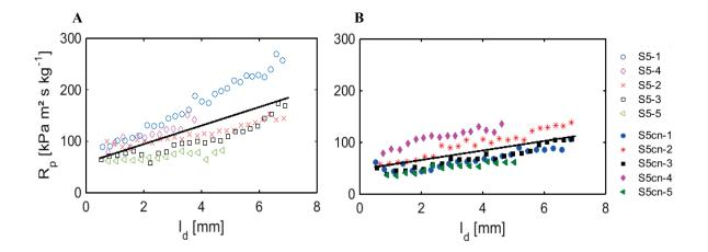
**Fig. 7:** Evolution of the product resistance with the dried layer thickness calculated from PRT data obtained in tests performed without stoppers and spontaneous nucleation (S5) (Fig. 6A) and PRT data obtained in tests performed without stoppers and with controlled nucleation (S5cn) (Fig. 6B). Symbols: experimental data; Solid line: fitting of the experimental data with Eq. (6).
