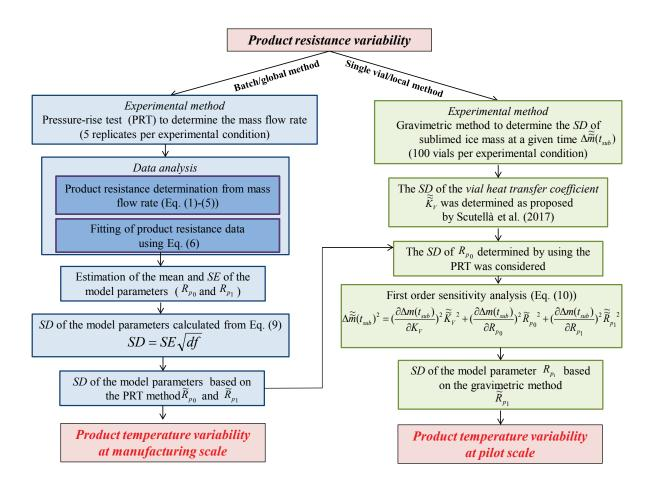
**Fig. 2:** Flow chart used to determine the product resistance variability using the pressure rise test (PRT) and the gravimetric methods. SD: standard deviation; SE: standard error.
