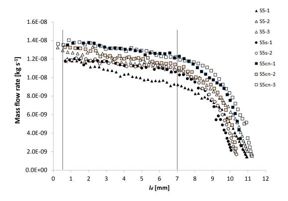
**Fig. 4:** Mass flow rates evolution as a function of the dried thickness in freeze-drying tests of 5 % sucrose solution processed in vials without stoppers and spontaneous nucleation (S5, triangles), with partially inserted stoppers and spontaneous nucleation (S5s, circles) and without stoppers and controlled nucleation (S5cn, squares). The mass flow rates were determined by the PRT method from Eq. (8). Vertical solid lines represent the mass flow rates data range considered in the analysis.
