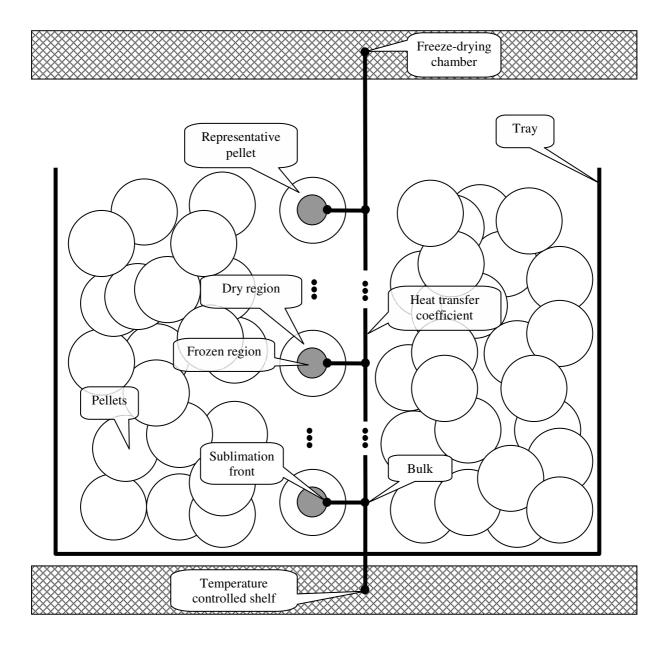
Figure 1. Schematic representation of heat transfer during freeze-drying of pellets.
